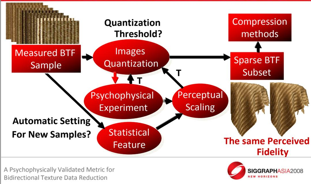
This fact motivated us try to develop a relatively simple technique for BTF data reduction outlined in this slide. We start with original data. We apply vector quantization of BTF images, but the question is how to set the optimal quantization threshold for each sample.
