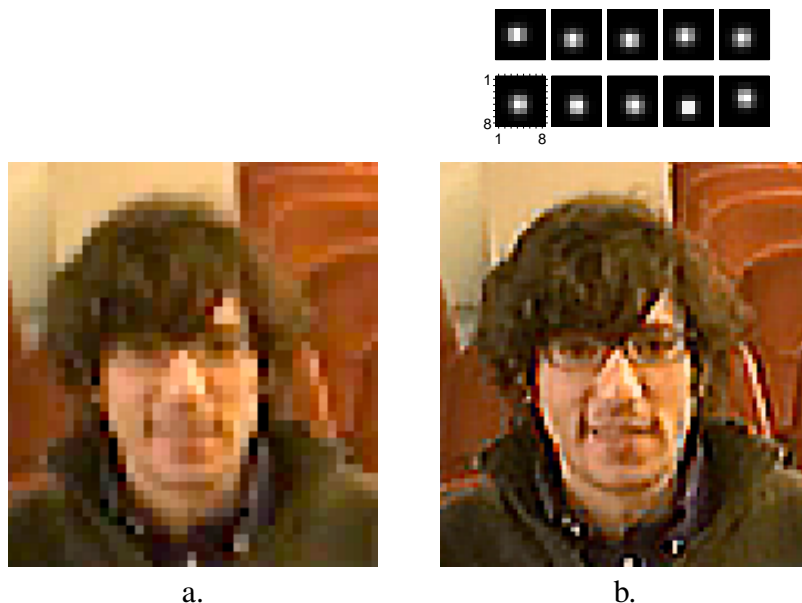
FIGURE 3. Reconstruction of images acquired with a webcam ( \epsilon = 2 ): (a) one of ten LR frames extracted from a short video sequence captured with the webcam, zero-order interpolation; (b) HR image and blurs estimated by the BSR algorithm. Note that many facial features, such as glasses, are not apparent in the LR image, but are well reconstructed in the HR image.
