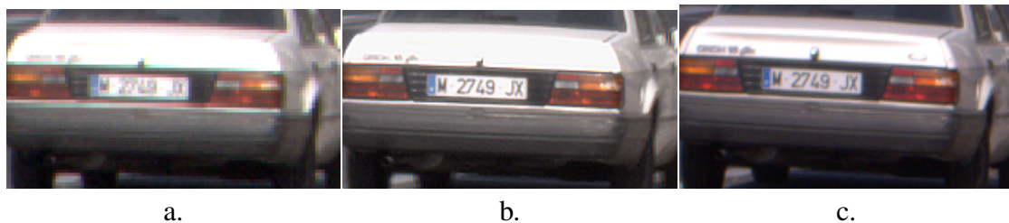
FIGURE 4. Reconstruction of images acquired with a digital camera ( \epsilon = 5/3 ): (a) one of eight LR images enlarged by zero-order interpolation; (b) HR image estimated by the BSR algorithm; (c) image acquired with optical zoom 1.7\times . The BSR algorithm achieved reconstruction comparable to the image with optical zoom.
