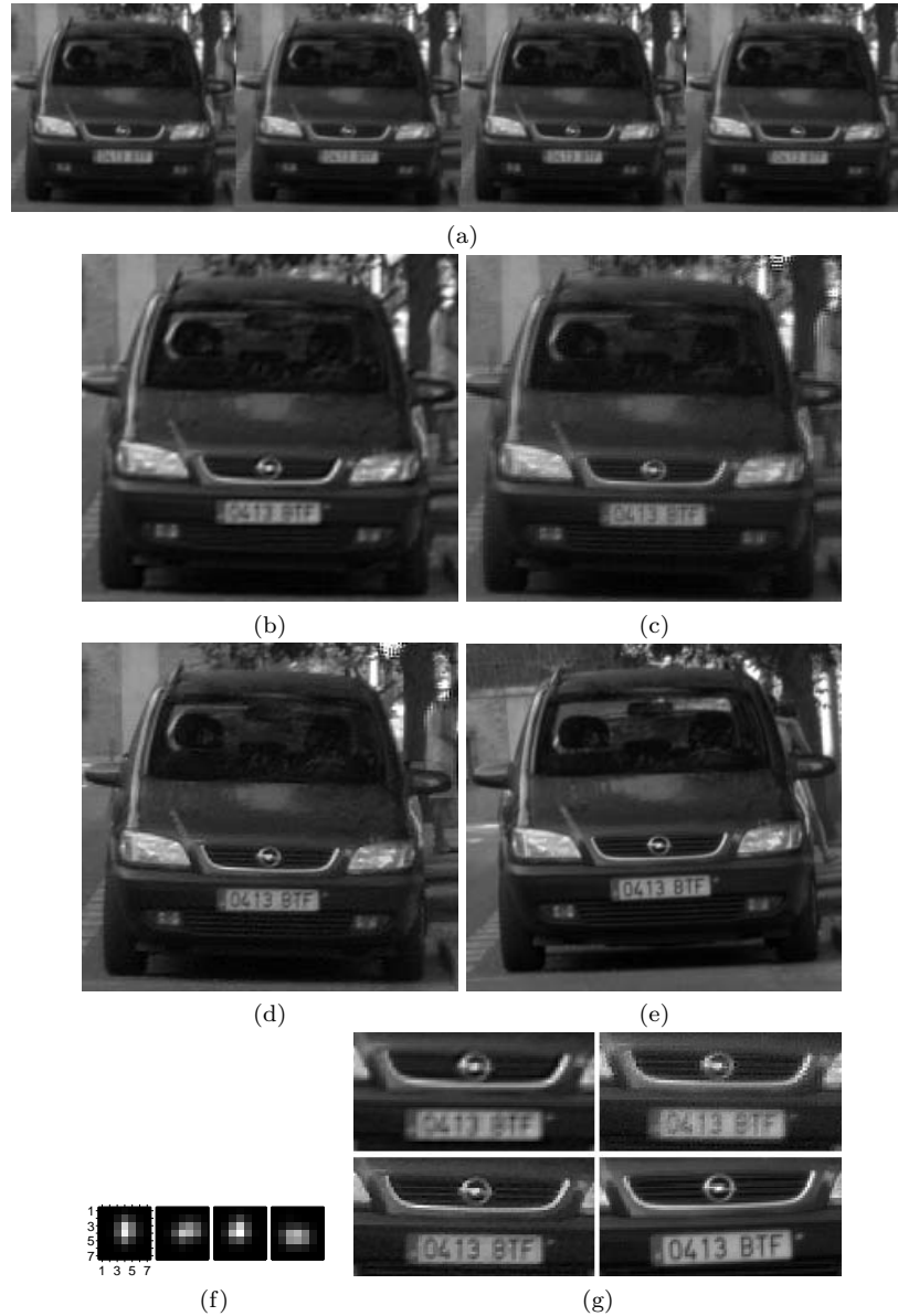
FIGURE 8.11: Reconstruction of images acquired with a digital camera ( \varepsilon = 5/3 ): (a) four LR images used in the reconstruction; (b) MBD followed by bilinear interpolation; (c) standard SR algorithm; (d–f) BSR algorithm showing the HR image together with recovered blurs; (e) image acquired with the camera mounted on a tripod and with optical zoom 1.7\times ; (g) close-ups of the results (b), (c) on top and (d), (e) on bottom. Due to blurring and insufficient resolution of the LR images, both MBD (b) and the standard SR method (c) give unsatisfactory results. Only the BSR algorithm (d) achieves reconstruction comparable to the image with optical zoom (e).
