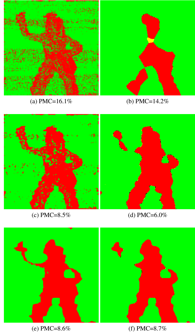
Figure 4: Two-plane decision maps: (a), (c) and (e) show results of maximum selection rule without averaging, with 3 \times 3 and 15 \times 15 averaging window, respectively; (b), (d) and (f) show results of the proposed segmentation approach with the initial DM from (a), (c) and (e), respectively.
