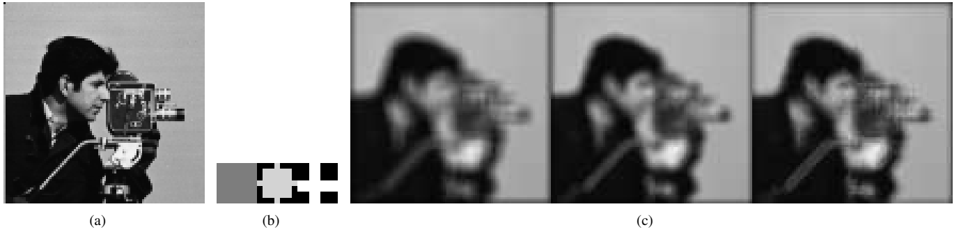
Fig. 1. (a) original 100 \times 100 cameraman image used for simulations; (b) three 7 \times 7 convolution masks; (c) blurred and noise-free images
